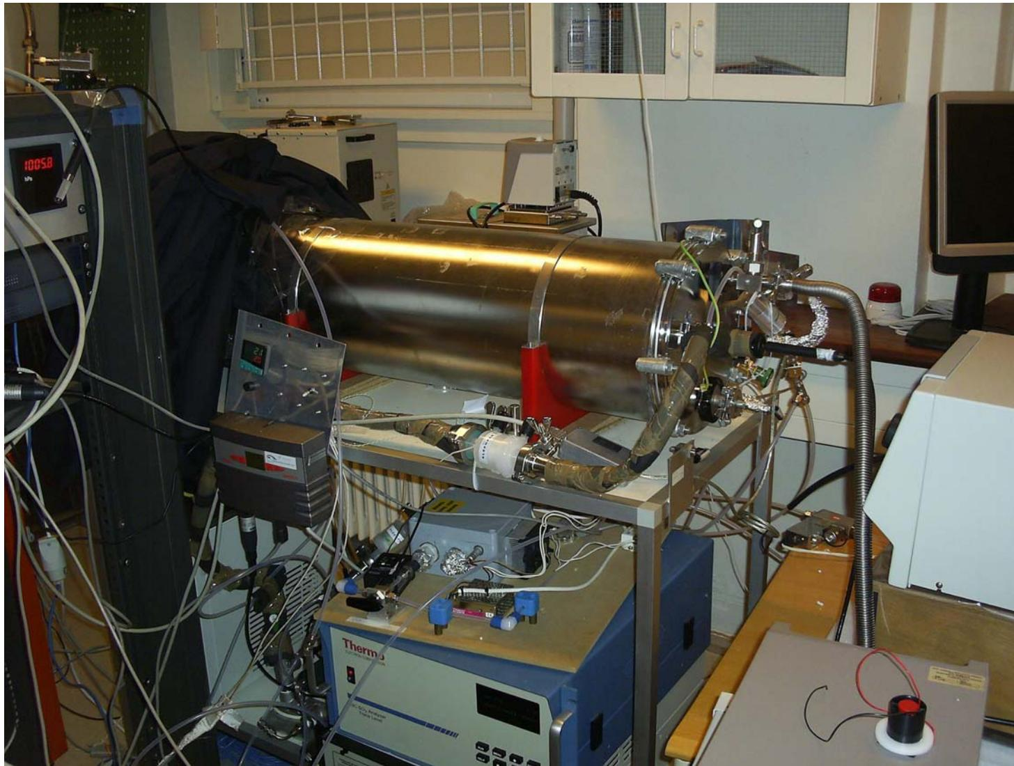
The chamber was cleaned carefully with nitric acid to remove surface contaminants
